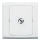
S1090 WHI ME 25A front flex outlet with 3 terminal block, each of which will accommodate up to 2nos. of 4mm 2 conductors
