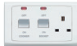
S5061 WHI ME Cooker connection unit 45A DP main switch & 13A SP switched socket with neons
